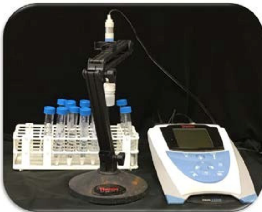
Figure 1. Fluoride ion selective electrode used for testing the concentration of fluoride.
