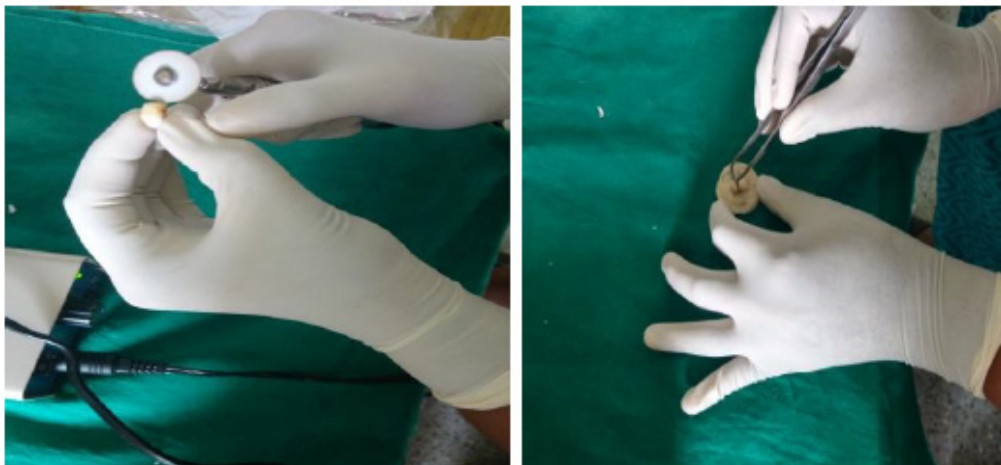
Figure 2. Specimen preparation using carborundum disc and mounting.
